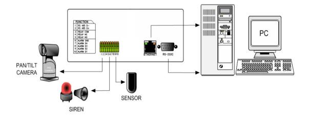
RS-232C : Control DVR through RS-232C port by using PC. RS-485 : Control external device like PTZ Camera RELAY Output : Relay Output SENSOR Input : SENSOR Input (Alarm connection) ETHERNET : Connection to LAN, WAN, Internet.
